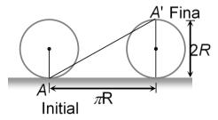
So the displacement of the point which was initially in contact with ground
