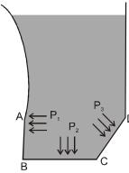
Let  $P_1$ ,  $P_2$  and  $P_3$  be the pressures exerted by the water on the wall AB, base BC and the wall CD respectively. Density of water is  $\rho$  and g is acceleration due to gravity. Then, approximately
