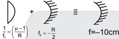
$$\frac{1}{f_1} = \left( \frac{\mu - 1}{R} \right) \quad f_2 = -\frac{R}{2} \quad f = -10 \text{ cm}$$
