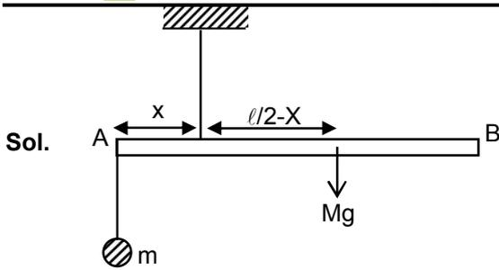
Balancing torque w.r.t. point of suspension
