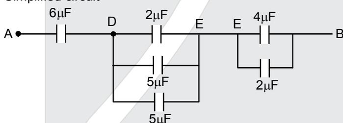
$$\frac{1}{C_{eq}} = \frac{1}{6} + \frac{1}{12} + \frac{1}{6} = \frac{5}{12} \Rightarrow C_{eq} = \frac{12}{5} = 2.4\mu\text{F}$$
