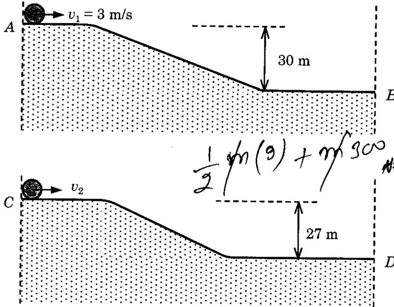
$$\frac{1}{2} m (v_1)^2 + m \times 30 = \frac{1}{2} (3m/R^2) \omega^2$$
