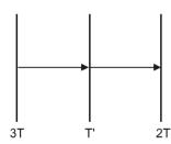
In steady state energy absorbed by middle plate is equal to energy released by middle plate.  $\sigma A(3T)^4 - \sigma A(T')^4 = \sigma A(T')^4 - \sigma A(2T)^4$
