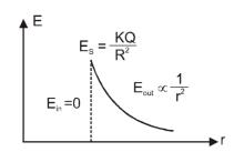
$V_{in} = \frac{KQ}{R} = constant$   $V_{out} = \frac{KQ}{r}$
