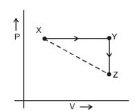
(A)  $\Delta S_{x\to z} = \Delta S_{x\to y} + \Delta S_{y\to z}$
