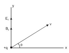
If  $\theta = 0^{\circ}$  then due to magnetic force path is circular but due to force  $qE_{0}(\uparrow)$  q will have accelerated motion along y-axis. So combined path of q will be a helical path with variable pitch so (A) and (B) are wrong.
