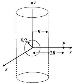
17. A cylindrical cavity of diameter a exists inside a cylinder of diameter 2a as shown in the figure. Both the cylinder and the cavity are infinitely long. A uniform current density J flows along the length. If the magnitude of the magnetic field at the point P is given by  $\frac{N}{12}\mu_0 aJ$ , then the value of N is
