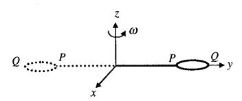
Now consider two similar systems as shown in the figure: Case (a) the disc with its face vertical and parallel to x-z plane; Case (b) the disc with its face making an angle of  $45^{\circ}$  with x-y plane and its horizontal diameter parallel to x-axis. In both the cases, the disc is welded at point P, and the systems are rotated with constant angular speed  $\omega$  about the z-axis.
