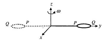
Now consider two similar systems as shown in the figure: Case (a) the disc with its face vertical and parallel to x-z plane; Case (b) the disc with its face making an angle of  $45^{\circ}$  with x-y plane and its horizontal diameter parallel to x-axis. In both the cases, the disc is welded at point P, and the systems are rotated with constant angular speed  $\omega$  about the z-axis.
