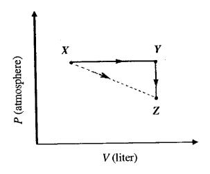
$$\Delta S_{x \to z} = \Delta S_{x \to y} + \Delta S_{y \to z}$$
