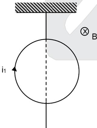
Restoring torque if given a small angular displacement =  $MB\sin\theta$ .
