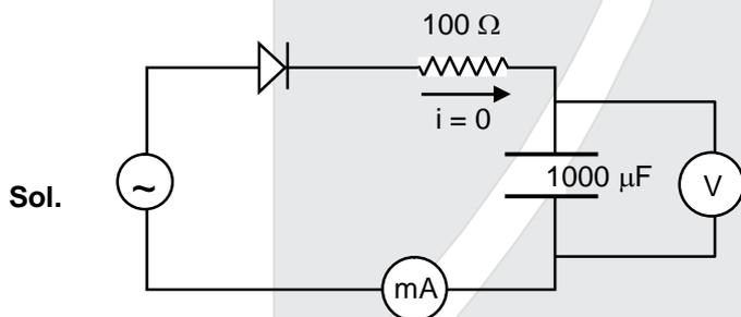
In this state the circuit will work as half wave rectifier and the voltage across capacitor will be equal to average value of voltage of ac source over a half cycle.
