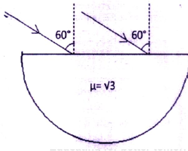
Is it possible that all the rays of this beam emerge from the spherical surface? (You may use  $\frac{1}{\sqrt{3}} \cong \sin 35^\circ$ )
