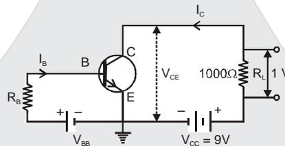
Sol. The circuit arrangement is shown in figure. Collector current,  $I_C = \frac{\text{Voltage drop across } R_L}{R_L}$
