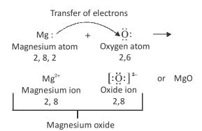
We find that the magnesium ion has 2 units of positive charge whereas the oxide ion has 2 units of negative charge. The oppositely charged magnesium ions, Mg<sup>2+</sup>, and oxide ions O<sup>2-</sup>, are held together by a strong force of electrostatic attraction to form magnesium oxide compound Mg<sup>2+</sup>O<sup>2-</sup> or MgO. Thus, magnesium oxide contains ionic bonds.
