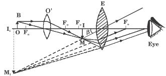
The object OB is placed just beyond the focus of the objective, which forms a real, inverted and magnified image. This image is formed within the focus of the eyepiece, which produces a virtual, erect and magnified image. The final image I<sub>1</sub>M<sub>1</sub> is adjusted to be formed at the least distance of distinct vision. The eyepiece acts as a magnifier.
