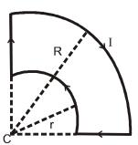
The permeability of free space is  $\mu_0$ . The magnetic field at C is (A)  $\mu_0 I(1/r - 1/R)/8$  into the page (B)  $\mu_0 I (1/r - 1/R)/8$  out of the page (C)  $\mu_0 I(1/r + 1/R)/8$  out of the page (D)  $\mu_0 I(1/r + 1/R)/8$  into the page
