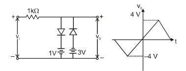
Assuming the diodes to be ideal, which of the following graphs depicts the output voltage  $v_0$  as function of time t ?
