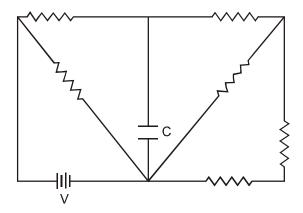
All the resistors are identical. The charge stored in the capacitor, once it is fully charged, is
