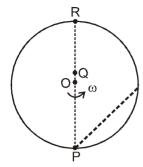
Since distance of particle P from point O is initially decreasing then increasing so, its angular velocity will initially increase then decrease. So, angle swept by P is more than angle swept by disc. So it will fall in unshaded portion.
