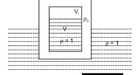
$$\rho_{c} (V_{0} - V_{i}) = \frac{V_{0}}{2} - V$$
