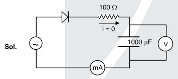
In this state the circuit will work as half wave rectifier and the voltage across capacitor will be equal to average value of voltage of ac source over a half cycle.
