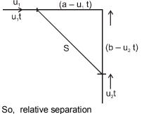
$$\begin{split} &S = \sqrt{\left(a - u_1 t\right)^2 + \left(b - u_2 t\right)^2} \\ &S = \sqrt{a^2 + u_1^2 t^2 - 2a \; u_1 t + b^2 + u_2^2 t^2 - 2b \; u_2 t} \\ &S = \left(a^2 + b^2 + \left(u_1^2 + u_2^2\right)t^2 - 2\left(au_1 + bu_2\right)t\right)^{\frac{1}{2}} \\ &So \text{ option (a) is correct} \end{split}$$
