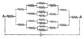
$R_{eq} \text{ between A and B}$  $= \frac{29R}{8}$
