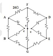
$$R_{DE} = 40/3 \ \Omega, \qquad R_{FDEG} = 160/3 \ \Omega,$$
