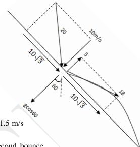
Thus the ball bounces with normal component 1.5 m/s and 'along plane' component  $3\sqrt{3}$  m/s.
