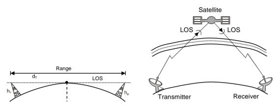
Figure. Space wave or line of sight LOS communication
